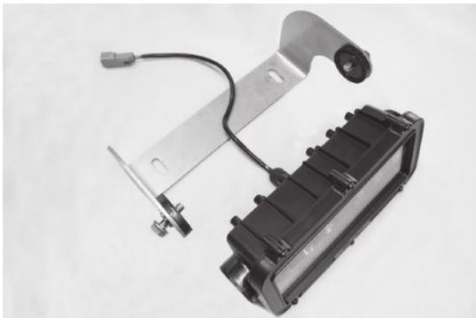
**2.** Install the lamp mounting bracket (B) on the Model 527 RED light using the two ratcheting plastic holders, four #6-19 x .357" screws and two M8-1.25x24MM hex bolts.
