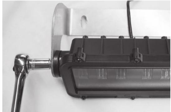
**5.** Align the lamp assembly, rubber damper (C) and the rock guard bracket (A), so that the rubber damper (C) is sandwiched between the lamp mounting bracket (B) and the rock guard bracket (A).
