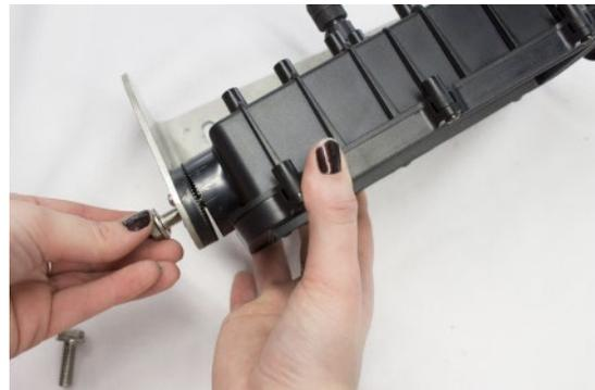
**3.** Rotate the Model 527 RED light in the ratcheting plastic holders to the desired light output angle.
