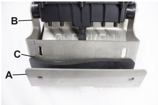
**6.** Route the Model 527 RED light power cord through the rock guard bracket access hole as shown.
