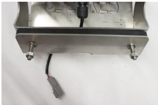
**8.** Use the tie wrap (D) to secure the lamp power cord to the rock guard bracket (A).
