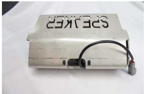
**7.** Use the two M10-1.5x40mm carriage bolts (F), M10 lock washers (E) and M10 hex nuts (G) to mount the complete assembly to the vehicle.
