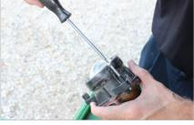
4. With the ball stud and light removed, insert the existing ball stud into the provided adapter bracket.
