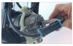
11. Plug in the connector on the other end of the wire harness into the tractor harness.
