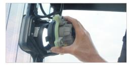
10. Plug in the provided wire harness into the back side of the new Model 90 headlight.
