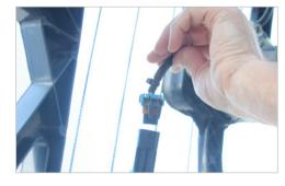
12. Adjust vertical aiming with the T20 Torx screwdriver on the exposed ball stud head on the front of the light assembly.
