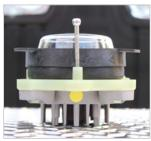
8. Using the T20 Torx screwdriver, turn each of the 2 remaining ball studs counter-clockwise seven full turns.
