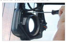
9. Line up the ball stud retainers in the provided adapter with the ball studs in the light housing on the grill. Snap into place. Check that the rubber boot is evenly seated around the light housing opening.
