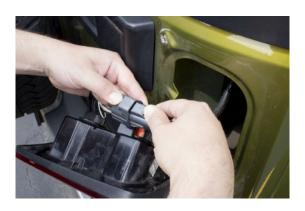
4. Feed the provided screws through the top of the resistor and attached the provided nuts by hand.
