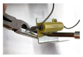
**5.** Use pages 2 and 4 of these instructions to line up and mark holes to drill for mounting the light. Once holes have been drilled, attach the bracket and resistor assembly to sheet metal on the vehicle. **NOTE:** Hardware for mounting the light to the vehicle is not provided.
