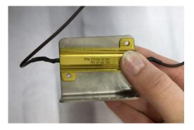
**3.** Secure the nut on the back of the resistor mounting bracket with a pair of pliers OR adjustable wrench, then tighten both screws with a Phillips screwdriver.
