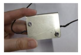
**4.** Align and attach the provided S-clips on resistor mounting bracket. The rounded edge should be on the same side as the resistor. Apply force until the S-clips fully engage.
