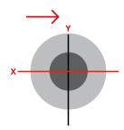
**9.** Repeat this process on the other headlight. Both headlights should match the diagram below, where the alignment point is even with the point where the X and Y axis crosses.
