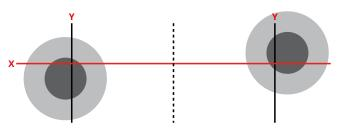
**7.** Using the alignment mechanisms in your vehicle, adjust one headlight vertically until the alignment point is even with the X axis.
