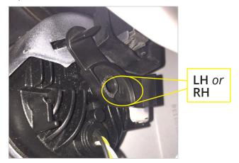
6. Insert the provided bolt into the back of the retaining bracket. Torque to 32 in-lbs to ensure proper tightening.
