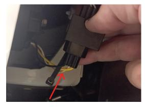
2. Loop the zip tie around the vehicle connector, passing through the wires. Close the zip tie to secure the two connectors.
