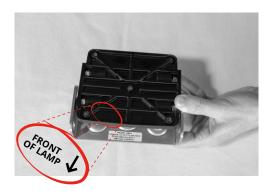
7. Align front of the headlight with "Front" text on the Mounting Base. Lamp will rock if not properly aligned. Attach Mounting Assembly to the headlight using the 4, 1/4"-20x0.75" Hex Head Flange Bolts. Tighten bolts to 46-50 IN-LBs.
