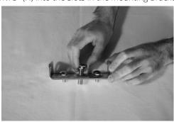
6. Attach the Mounting Bracket (D) to the Mounting Base (A) with the 4, M8-1.25"x25 Hex Head Flange Bolts (F). Tighten the bolts by hand. These combined parts are the Mounting Assembly.
