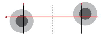
**8.** On the same headlight, adjust the same headlight horizontally until the alignment point is even with the Y axis.
