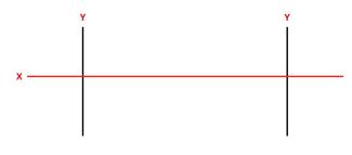
The goal of this sheet is to aim BOTH of your headlights so that the **Alignment Point** is at the crossection of the horizontal X and vertical Y lines you have drawn. The following directions illustrate the process and proper aiming of headlights.
