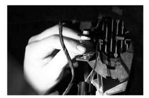
**12.** Insert the adjustment screw from the bottom of the aligned adjustment arms, through the spring, into the plastic nut. Turn the adjustment screw until it engages the plastic nut. Compare the pattern of the light coming from the 2 fog lamps as the shine on the wall by covering and uncovering each lamp individually.
