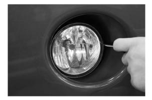
**2.** Using the #2 Phillips screwdriver or socket wrench, carefully remove the adjustment screw. Pull out and discard the springs and screw.
