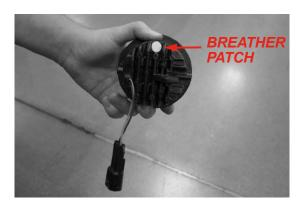
**6.** Feed the wire on the **BACK** of the light through the mounting bucket and orient the plastic mounting bucket with the "TOP" text at the TOP of the light.
