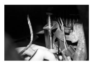
**3B-1: PASSENGER SIDE:** Facing the front of the vehicle, locate the mounting tab on the **LEFT** side of the stock fog light. Use the flat blade screwdriver to depress the mounting tab until the post is released from the mounting tab.
