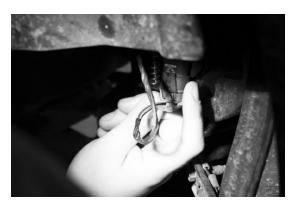
**3A-1. DRIVER SIDE:** Facing the front of the vehicle, locate the mounting tab on the **RIGHT** side of the stock fog light. Use the flat blade screwdriver to depress the mounting tab until the post is released from the mounting tab.
