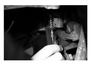
**3A-2.** Using one hand at the front and one at the back of the light, wiggle the stock fog light free from the shroud. Caution: If you depress the LEFT side first, the light will get stuck. Avoid applying excessive force as it may break off the mounting tab inside the shroud.
