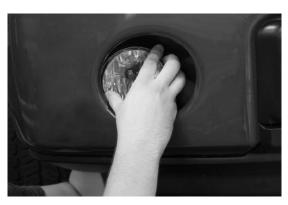
**5.** Holding the J.W. Speaker lights face-down, orient them so that the breather patch is at the **TOP** and the wiring is on the **LEFT**.
