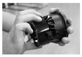
9. Guide the **LEFT** post on the mounting bucket into the mounting tab on the shroud. Once inserted, push the **RIGHT** post into place. The light should pivot freely up and down (about 10 degrees).
