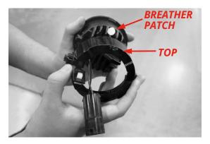
8: Take the light with the "TOP" text on top (when looking at the light from the back), and feed the wires through the hole in the shroud. Ensure that the "SPEAKER" logo is right-side up across the bottom of the front of the light. Caution: If installed incorrectly, the light pattern will be upside-down and will NOT be street legal.
