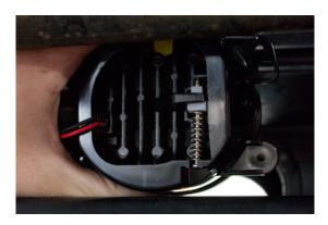
8. Rotate the adjustment screw (clockwise to raise, counterclockwise to lower) on the rear of the lamp to aim the light like the existing fog light.
