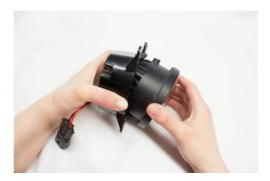
6. Hold the lamp assembly into the bumper. Use the 4 mounting holes to align it into position.
