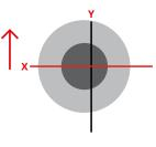
**9.** Repeat this process on the other headlight. Both headlights should match the diagram below, where the alignment point is even with the point where the X and Y axis crosses.
