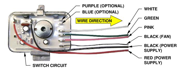
Disassemble switch circuit from back cover (2 screws, 2 lock washers and 2 nuts).
