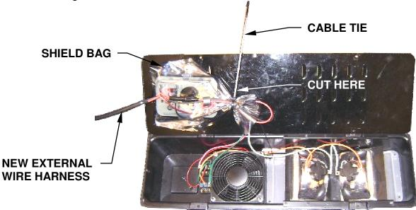
Cut off excess cable tie (do not puncture bag) and reassemble back cover onto lamp fan assembly.
