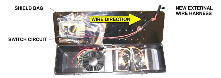
Note: Must route screws through holes in static shielding bag and switch circuit. Do not tear or puncture static shielding bag.
