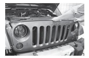
**5.** Use a T15 Torx driver to remove the 4 screws holding the headlight retaining ring. **Save the 4 screws.**
