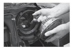
**10.** Re-attach the retaining ring. Align all 4 tabs on the ring with the screw holes. It will only fit in one orientation. Install 4 screws from step 5 using the T15 Torx driver.
