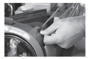
**3. Carefully** remove the front grill by pulling the **TOP** portion forward until it unsnaps. Start near one headlight and work across to the other light.
