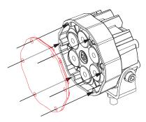
**2.** Place the outer bezel (#2) on the lamp over the lens. Be sure the J.W. Speaker logo on the outer bezel is oriented at the bottom of the lamp.
