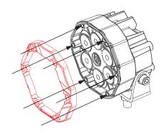
**3.** Take 6 of the M4 bezel screws (#1), place them in the holes of the outer bezel, and fasten the lens and bezel to the light using the T20 Torx Wrench. Repeat steps 1-3 on the light.
