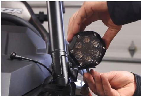
**5.** Aim the Trail 6 as desired and fasten the side bolts (#5) using 5mm Hex Key. Plug in the provided harness into the back of the lamp.
