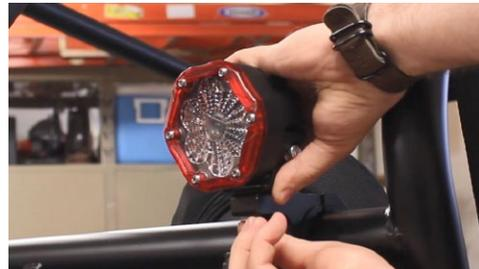
12. Aim the Trail 6 as desired and fasten the side bolts (#5) using 5mm Hex Key. Plug in the provided daisy chain harness into the back of the lamp.
