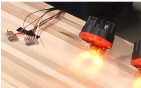
6. The parent lamp has a single flash x 5 times for low sensitivity, 2 flashes x 5 times for medium sensitivity, and 3 flashes x 5 times for highest sensitivity. Once it is at the sensitivity you want disconnect the green wire and it will save that setting to the lamp. Cap the green wire.
