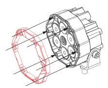
**3.** Take 6 of the M4 bezel screws (#1), place them in the holes of the outer bezel, and fasten the lens and bezel to the light using the T20 Torx Wrench. Repeat steps 1-3 on the other light.
