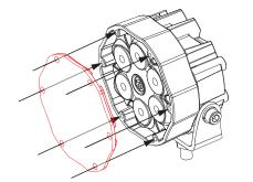
**2.** Place the outer bezel (#2) on the lamp over the lens. Be sure the J.W. Speaker logo on the outer bezel is oriented at the bottom of the lamp.
