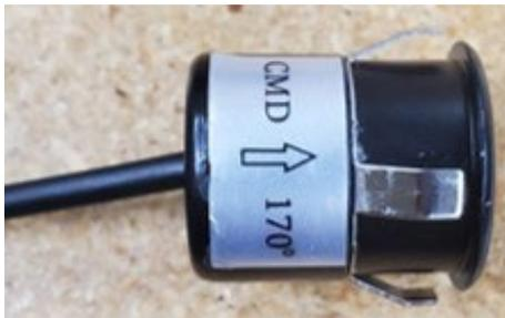
5. Determine how you want the bezel mounted on the Trail 6. Next put the camera wire through the mount and ensure the arrow (top of the camera) is facing up.
