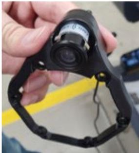
6. Ensure the arrow (top of the camera) is facing up. Snap Camera into the bezel by applying pressure.
