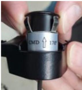
7. **FLUSH MOUNT ONLY:** Secure the camera wire by pressing it into the wire routing channel on the bezel.
