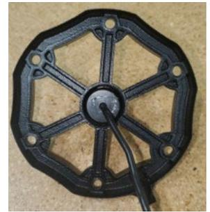
11. Insert the tips of the needle nose pliers into the 2 small holes on the back of the camera. Then turn only in the clockwise direction to aim the camera.
