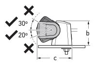
Dimensions: a = 350mm / 13.78" b = 56mm / 2.20" c = 81mm / 3.19" d = min. 200mm / 7.87" max. 280mm / 11.02"
