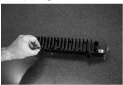
5. Attach 1/4-20 mounting bolts through rear hole of bracket into the hex nuts
