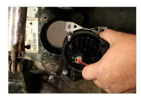
5. Plug in the connector, making sure the locking tab engages.
