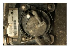
2. Disengage the locking tab on the connector to remove it from the factory light.
