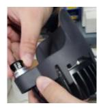
6. Connect camera to monitor. AV1 connects to the driver's side light, and AV2 connects to the passenger's side light.
