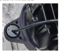
9. Insert the tips of the needle nose pliers into the 2 small holes on the back of the camera while it is **installed on the lamp**. Then turn only in the clockwise direction to aim the camera.
