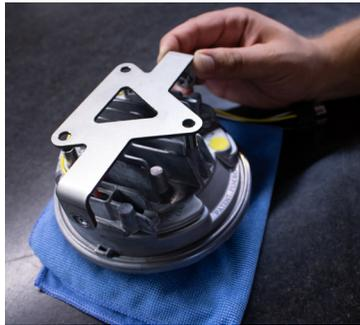
8. Take your J.W. Speaker lamp and place it face down on the lens on a protected surface so the lens does not get scratched. Put the rubber ring around the housing of the light.
