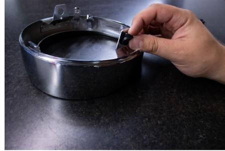
5. Remove the lamp assembly from the trim ring. the lamp assembly can only be removed by sliding it out of the ring, lens forward.
