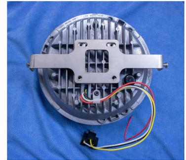
8. Take your J.W. Speaker lamp and place it face down on the lens on a protected surface so the lens does not get scratched. Put the rubber ring around the housing of the light.
