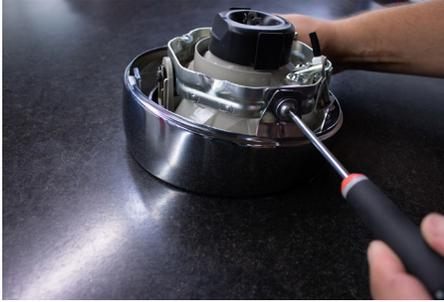
6. Remove the rubber grommets in the trim ring.
