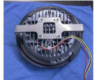
9. Place the lamp/ bracket assembly in the trim ring. Place the M5 bolt through the trim ring, and into the JWS bracket. Tighten the M5 bolt with the appropriate hex wrench.
