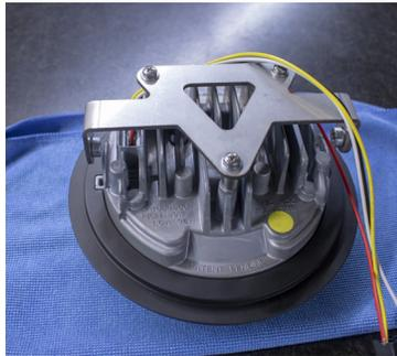
9. Place the lamp/ bracket assembly in the trim ring. Take the M5 bolt, bushing, and the lock washer, and assemble them as seen in photo. Tighten the M5 bolt with the appropriate hex wrench.
