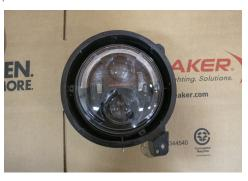
**5.** Connect the mounting ring over the headlight to secure the headlight into the bucket. Use the SHORTER Philips screws (x3) to secure the mounting ring.
