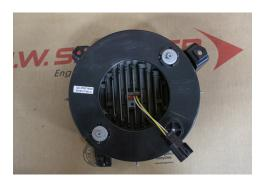
**10.** After you have the headlight pattern properly aimed, remove the headlights again and to tighten the 3 bolts on the bucket. This will prevent the new headlights from shaking and vibrating. **Be careful to not over or under tighten the bolts.**
