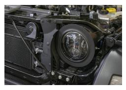
**9.** With both headlight kits assembled and mounted onto the front housing of your Jeep. You are ready to aim your headlights. Aim the new headlights to the same height as the original beam pattern that you marked before we started this install. This is done by turning the vertical adjuster with a Philips screwdriver. (Located on the top of the housing)
