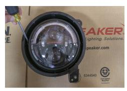
**6.** Mount the Bezel on the bucket by aligning the slots on the outside perimeter of the bucket with the screw holes. Push down on the bezel to get them aligned. Secure the bezel by using the LONGER Philips screws (x4).
