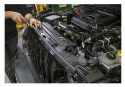
**2.** Take out the old halogen headlights by loosening the 10mm bolts (x3). Once the bolts are loose, the entire housing can be removed from the vehicle and the wire adapter can be unplugged.
