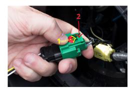
**8.** Plug in the new LED headlight remembering to plug in the turn signal as well. Use only the wire harness provided. Then install it into the mounting ring.
