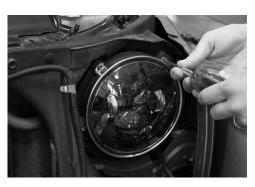
**6.** Remove the retaining ring and headlight from the mounting ring. Box" are present and complete.
