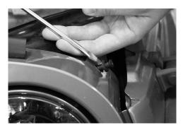
**3.** Carefully remove the front grill by pulling the **TOP** portion forward until it unsnaps. Start near one headlight and work across to the other light.
