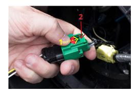
**8.** Plug in the new LED headlight remembering to plug in the turn signal as well. Then install it into the mounting ring. **NOTE:** On ECE versions, connect the BLUE wire for DRL.
