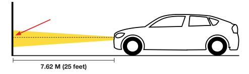
**Fog Lights** should be aimed so the top of the beam is about 4 inches BELOW the level line of the lights.
