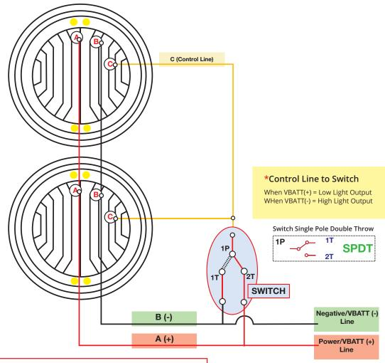
\* Control line must be connected to power V<sub>+</sub> or Ground V<sub>-</sub> At powerup of lamp, **control line** *cannot* **be floating** (Not connected)!
