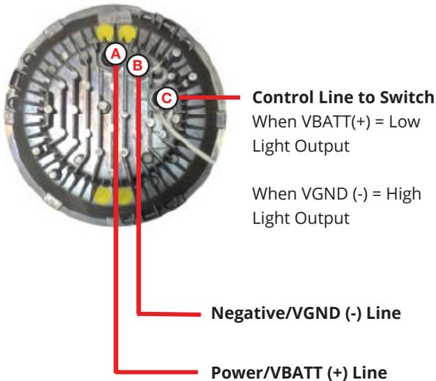
**Auxiliary/Ditch Light Wiring**
