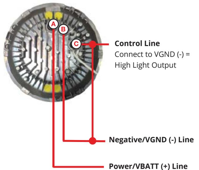
\* Control line must be connected to power  $V_+$  or Ground  $V_-$ .
