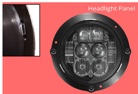
Figure 4: Slide the headlight into the mounting ring. Make sure the alignment tabs seat in the ring slots (see inset). Use the Speaker logo or regulatory printing to verify proper orientation.
