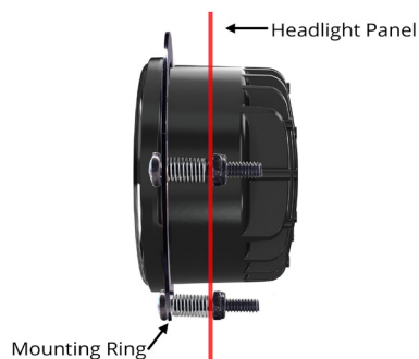
Figure 7: Tighten the three Torx screws until the springs are compressed approximately halfway. If there is an obstruction, back out all three screws about 1/4 inch.
