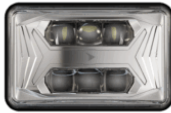
Part Number 0562031 12-24V DOT/ECE LED RHT Asymmetric Low Beam Headlight with Chrome Bezel
