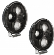
Part Number 0551693 12-24V ECE LED High Beam with Black Inner Bezel & Pedestal Mount - 2 Light Kit
