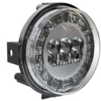
Part Number 0558361 12-24V DOT LED Low Beam/Front Position Headlight w/ Built in Turn Signal & Adjustable Mount
