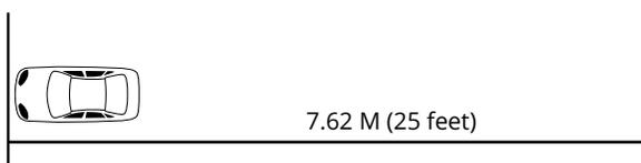
**2.** On the wall, draw a line from the ground to the approximate center point of the headlight. Repeat for the other headlight. This will create your Y axis lines.
