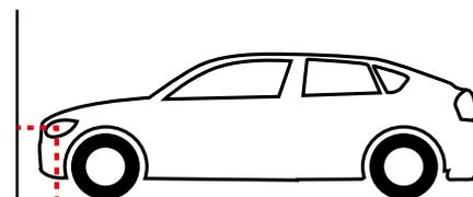
3. Connect the center points between headlights in a straight line, using chalk or tape. This will create your X axis (horizontal) line.
