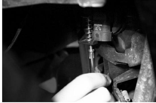
**3A-1. DRIVER SIDE:** Facing the front of the vehicle, locate the mounting tab on the **RIGHT** side of the stock fog light. Use the flat blade screwdriver to depress the mounting tab until the post is released from the mounting tab.
