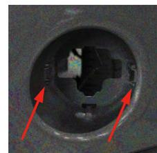
**Mounting Tabs:** The tabs located on either side of the shroud where the posts snap into place.
