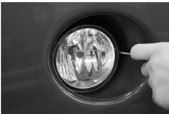
**3B-2:** Using one hand at the front and one at the back of the light, wiggle the stock fog light free from the shroud.
