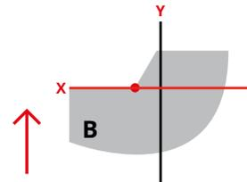
8. On the same headlight, adjust horizontally until the **Alignment Point** is even with the Y axis.
