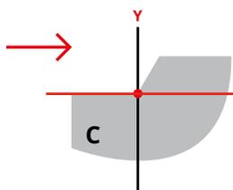
9. Repeat this process on the other headlight. Both headlights should match the diagram below, where the **Alignment Point** is even with the point where the X and Y axis crosses.
