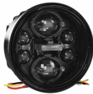
Part Number 0549871 12-24V DOT/ECE LED High Beam Headlight
