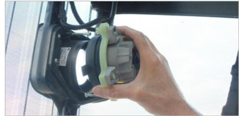
10. Plug in the provided wire harness into the back side of the new Model 90 headlight.
