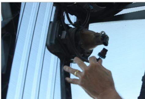
2. Pull to remove the existing headlight from the ball studs. Remove the existing rubber boot.
