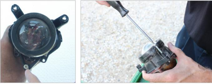
4. With the ball stud and light removed, insert the existing ball stud into the provided adapter bracket.
