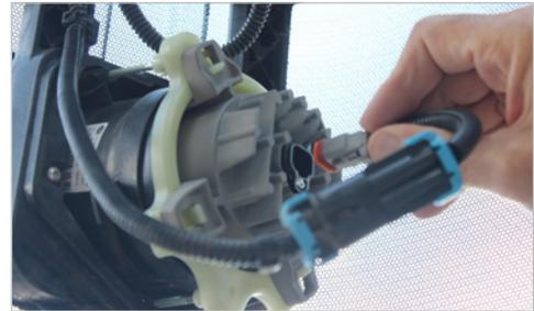
11. Plug in the connector on the other end of the wire harness into the tractor harness.
