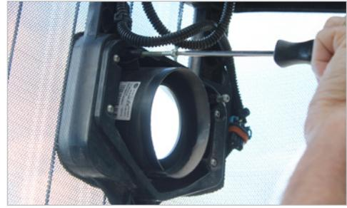
9. Line up the ball stud retainers in the provided adapter with the ball studs in the light housing on the grill. Snap into place. Check that the rubber boot is evenly seated around the light housing opening.
