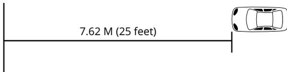
The goal of this sheet is to aim **BOTH** of your headlights so that the **Alignment Point** is at the crosssection of the horizontal X and vertical Y lines you have drawn. The following directions illustrate the process and proper aiming of headlights.
