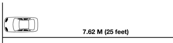
2. On the wall, draw a line from the ground to the approximate center point of the headlight. Repeat for the other headlight. This will create your Y axis lines.
