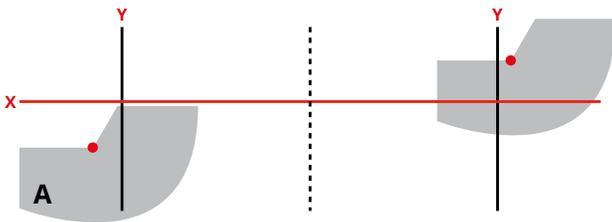
7. Using the alignment mechanisms in your vehicle, adjust one headlight vertically until the **Alignment Point** is even with the X axis.
