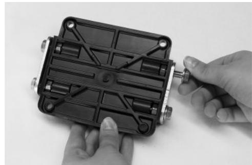
7. Align front of the headlight with "Front" text on the Mounting Base. Lamp will rock if not properly aligned. Attach Mounting Assembly to the headlight using the 4, 1/4"-20x0.75" Hex Head Flange Bolts. Tighten bolts to 46-50 IN-LBS.
