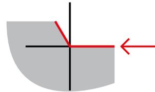
**Alignment Point:** The center of the angle in the Kink that must align to the center point when aiming the light at a wall.
