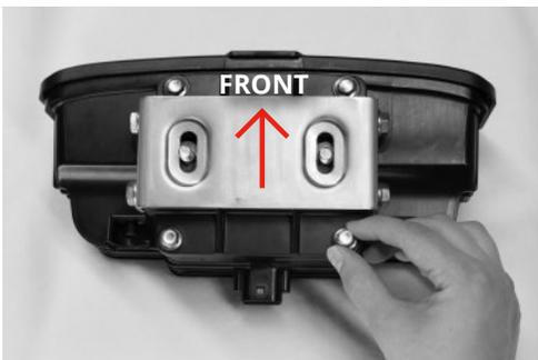
8. Mount headlight to the vehicle using the 2, M8-1.25"x25 Carriage Bolts (E), 2 M8 Split Lock Washers (G) and remaining 2 Hex Nuts (B). Carefully splice the wires using the "Wire Functions" and "Voltage" information from page 1 to power the light.
