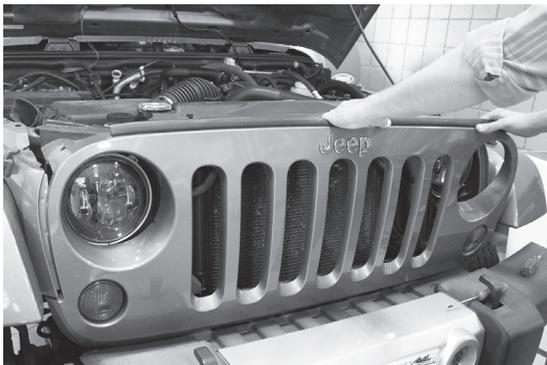
4. **Carefully** unsnap the clips at the bottom of the grill and let it rest across the bumper. **NOTE:** These clips may break if not treated with care.
