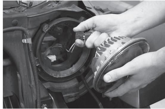
9. Align the alignment lugs on the lamp with the slots in the ring. The lamp will only fit in one orientation, and from the front the "Evolution J" text should be readable at the top.
