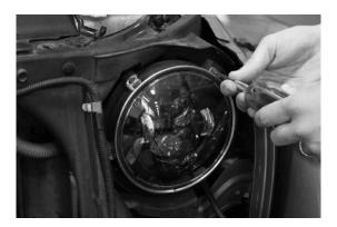
2. Carefully remove the 6 fasteners by prying them up at the base using a flat blade screw driver. Save the 6 fasteners.
