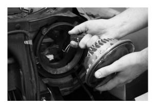
**10.** Re-attach the retaining ring. Align all 4 tabs on the ring with the screw holes. It will only fit in one orientation. Install 4 screws from step 5 using the T15 Torx driver.
