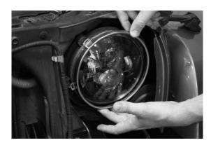
7. Unplug the existing headlight. NOTE: On newer models there is (1) a red button on the plug that must be pushed up, and (2) a green button that must be pressed and held to unplug the existing lamp.
