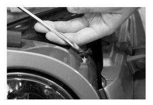
4. Carefully unsnap the clips at the bottom of the grill and let it rest across the bumper. NOTE: These clips may break if not treated with care.
